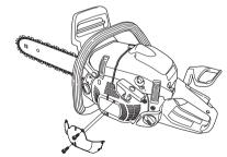
CAUTION! If the special winterising kit has been fitted or any measures have been taken to increase the temperature these changes must be reversed before the machine is used in normal temperature conditions. Otherwise there is a risk of overheating, resulting in severe damage to the engine. IMPORTANT! Any maintenance other than that described in this manual must be carried out by your servicing dealer (retailer).
